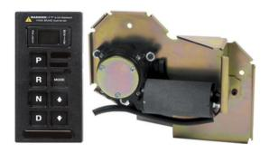
Up to seven buttons are available on the Shift By Wire Controller, giving vehicle OEMs a wide range of control over Transmission or ancillary functions. The MODE Buttons gives direct control over critical functions including a Power Take Off from the truck engine.
