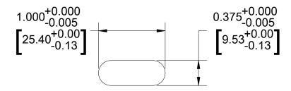
6300 and 6400 series switches mate with .108 and .170 thick panels 6301 and 6401 series switches mate with 2mm and 5mm thick panels Panel thicknesses include paint, overlays, decals and any other coverings A square edge is required on the wing retention side of the mounting slot
