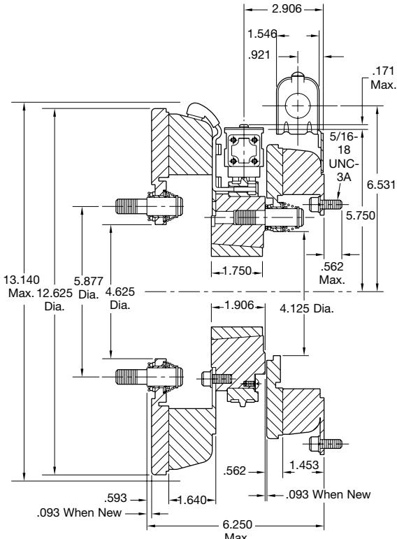
\* Mounting holes are within .010 of true position relative to pilot diameter.
