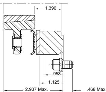
**Outside Mounted Flush Backing Plate**
