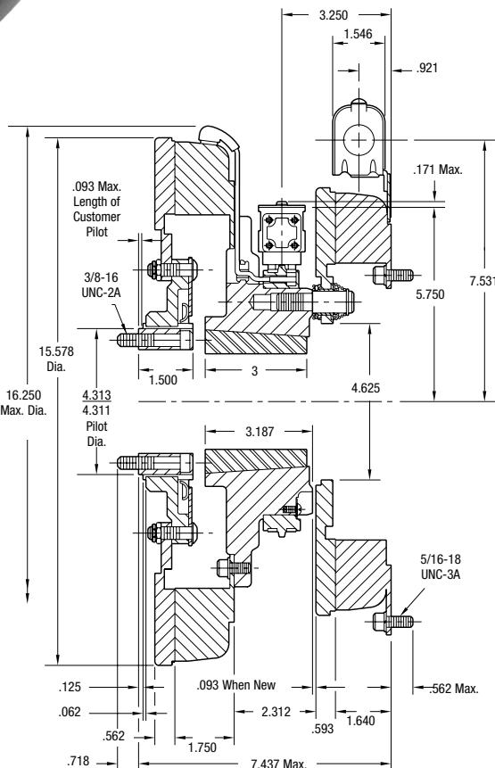
\* Mounting holes are within .010 of true position relative to pilot diameter.
