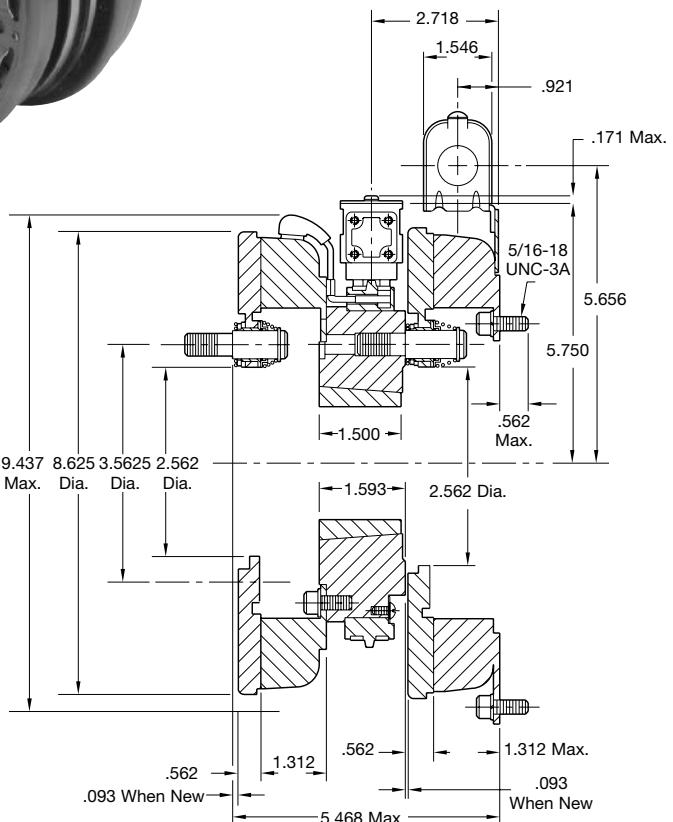
\* Mounting holes are within .010 of true position relative to pilot diameter.
