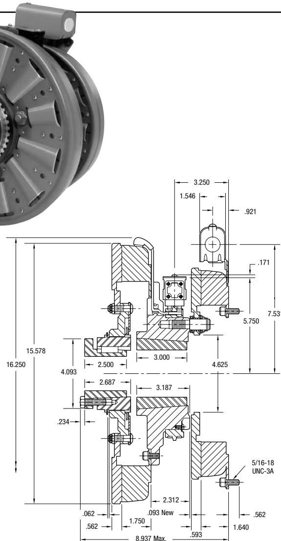
\* Mounting holes are within .010 of true position relative to pilot diameter.
