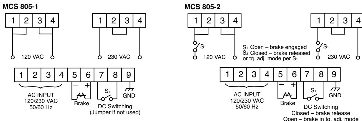
For AC switching, switch may be in series with input supply.
