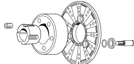
Torque is transmitted through three or four drive pins. Proven standard of the industry for all normal duty applications. Standard on clutches, brakes, motor brakes and clutch-brakes, size 500 to 1525.
