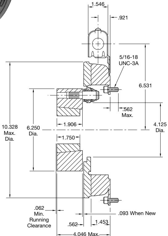
\* Mounting holes are within .010 of true position relative to pilot diameter.
