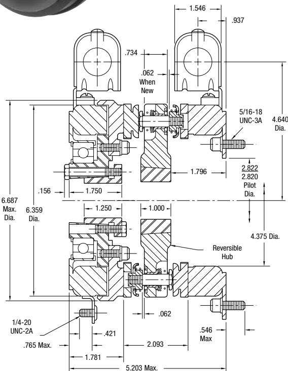
\* Mounting holes are within .010 of true position relative to pilot diameter.
