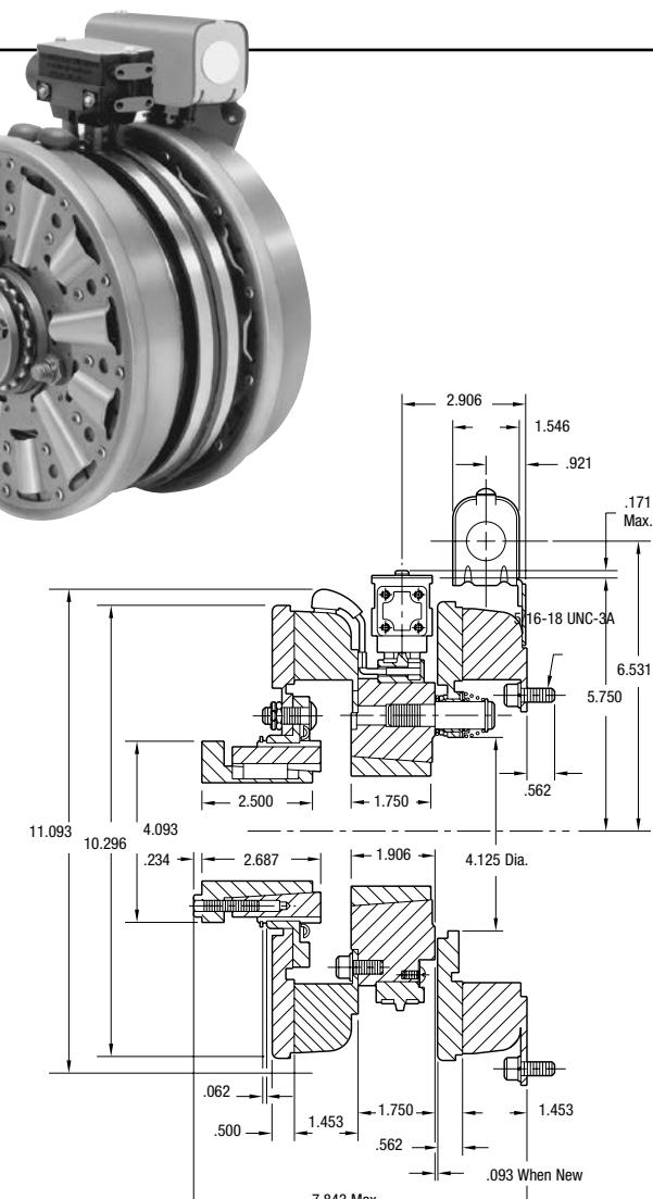
\* Mounting holes are within .010 of true position relative to pilot diameter.
