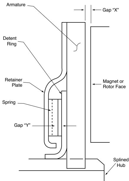
This can happen with excess vibration or mishandling. To reset the autogap, move the armature assembly toward the magnet or rotor. This can be done by 1) or 2) below:
