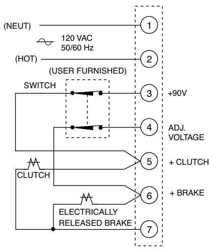
Clutch/Electrically Released Brake Operation
