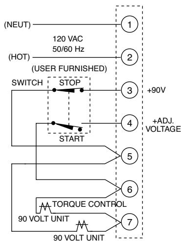
Normal Clutch/Brake Operation
