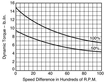
**Size 500-PC/PB**      Maximum Speed 5,400 rpm
