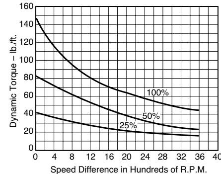
**NOTE:** Torque values are in inch lbs. for size 400 and smaller, and in ft.lbs. for size 500 and larger.
