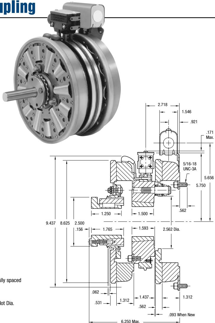
\* Mounting holes are within .010 of true position relative to pilot diameter.
