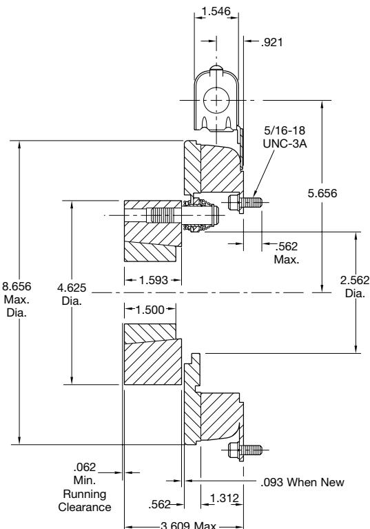
\* Mounting holes are within .010 of true positioning relative to pilot diameter.
