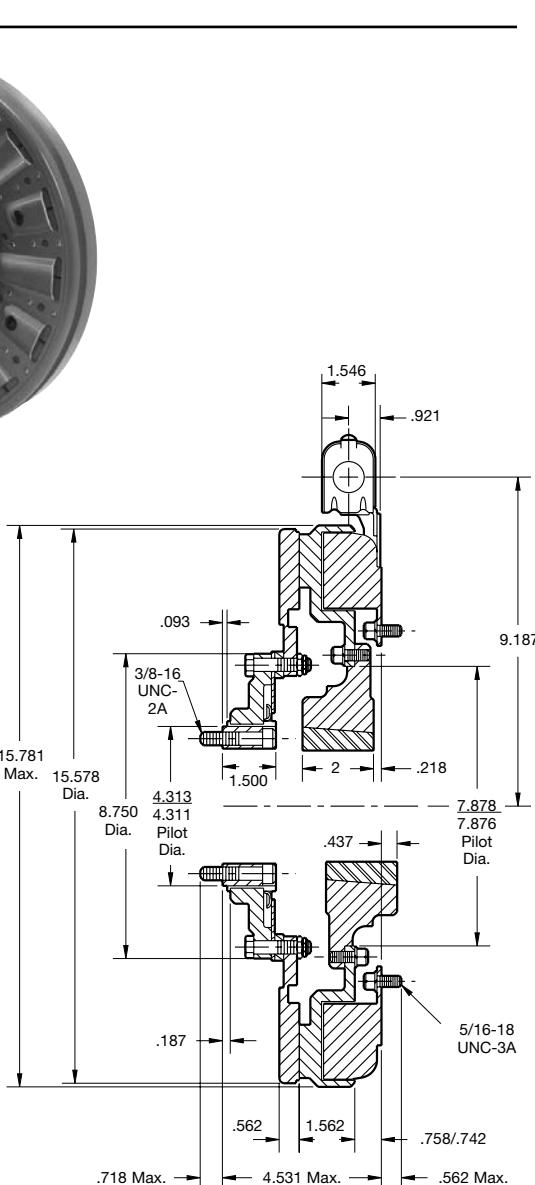
\* Mounting holes are within .010 of true position relative to pilot diameter.
