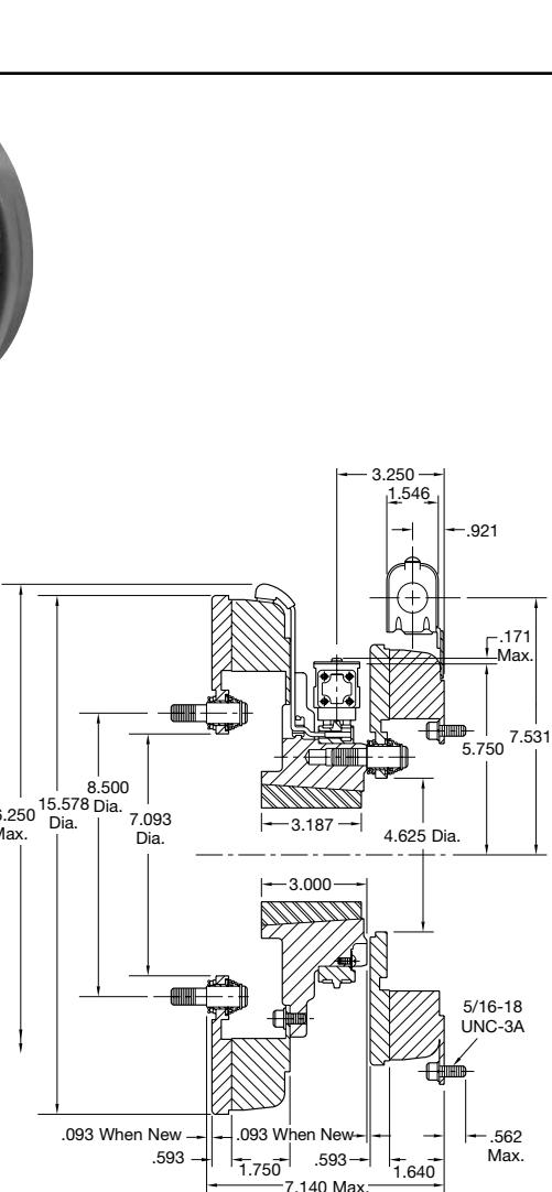
\* Mounting holes are within .010 of true position relative to pilot diameter.
