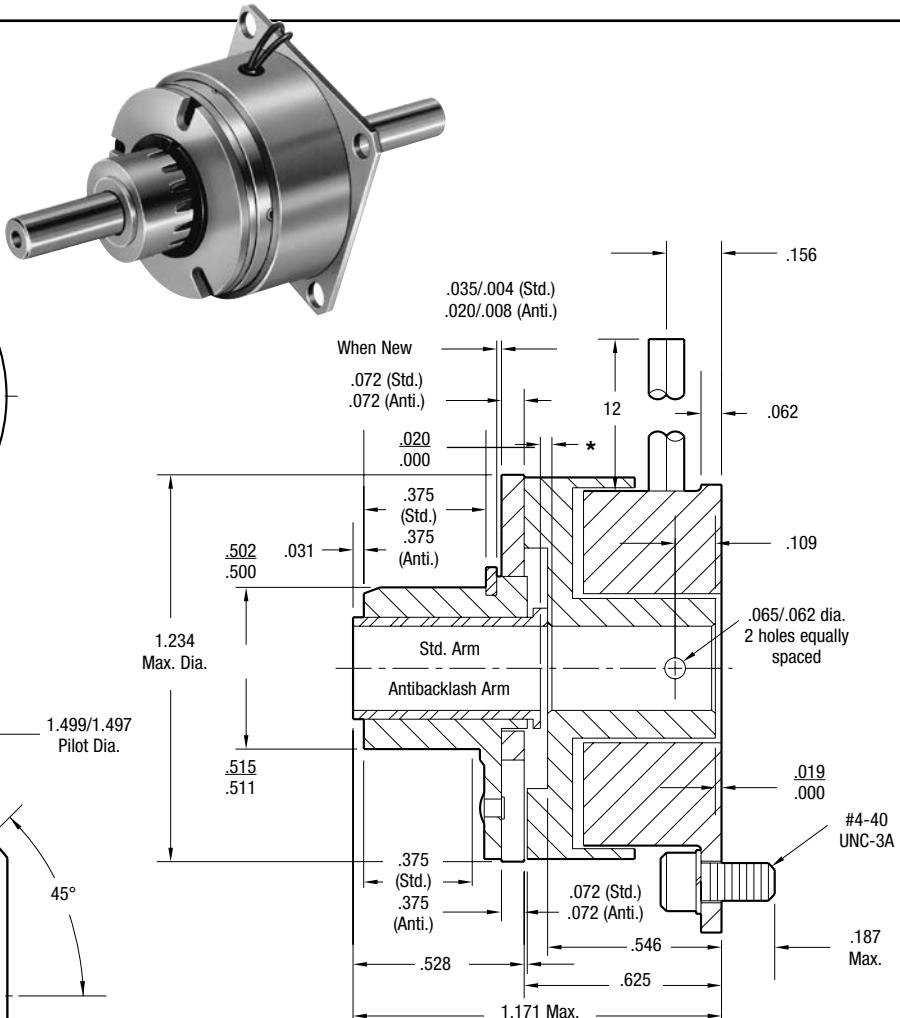
\* Mounting holes are within .006 of true position relative to pilot diameter.
